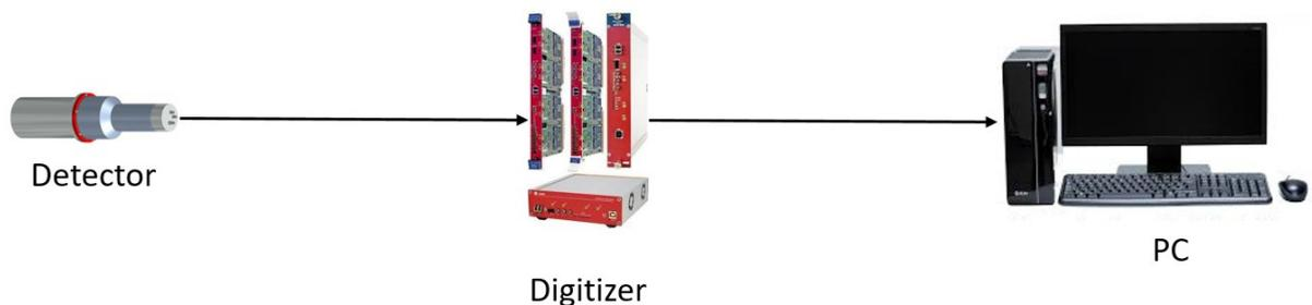
**Figure 5.** PMT – digitizer – PC connection
