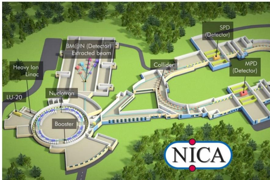
Figure 1 - Schematic view of the NICA accelerator complex[4]
