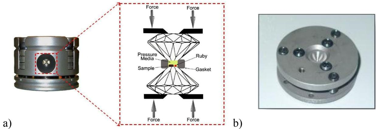
**Figure 5:** Schematic (a) and general view (b) of the diamond anvil cell [9]
