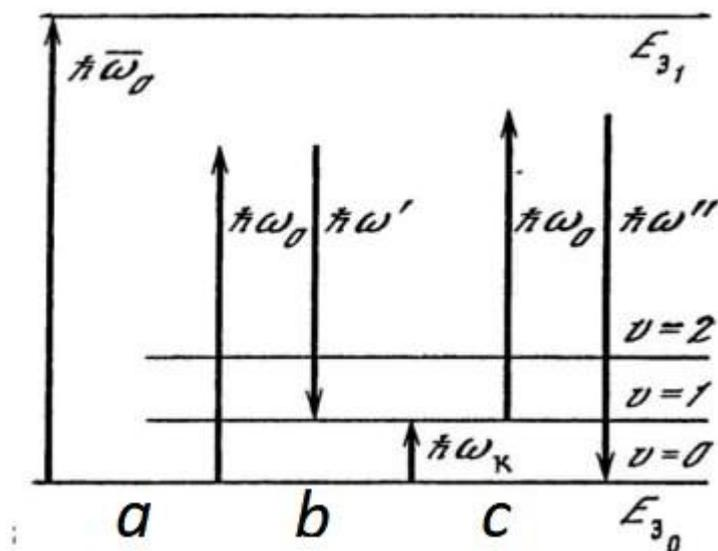
**Figure 2:** Schematic of transitions in absorption and Raman scattering of light [7]
