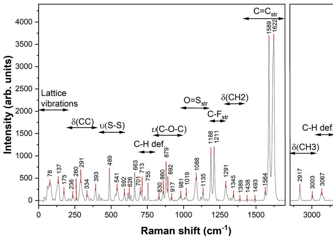
**Figure 6:** Raman spectrum of sulindac at room temperature and normal pressure
