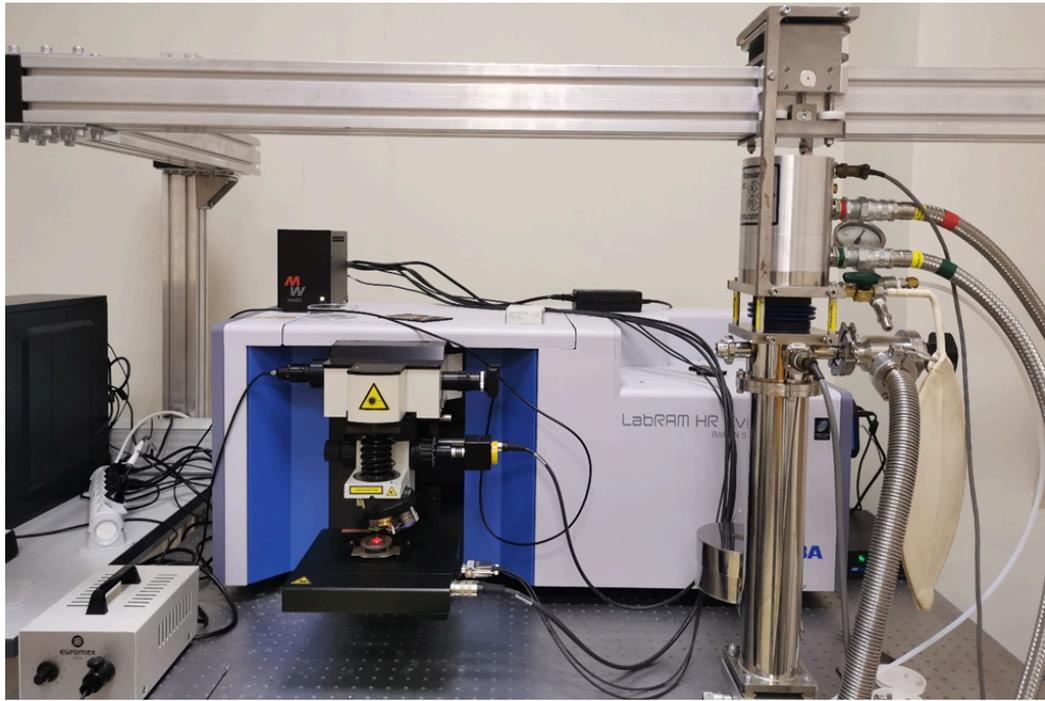
**Figure 4:** General view of the LabRAM HR Evolution Raman spectrometer (Horiba, France)
