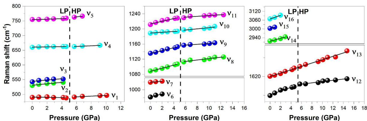
**Figure 8:** Pressure dependence of the frequencies of selected vibrational modes of the ambient and pressure-induced form-HP of the sulindac on pressure.
