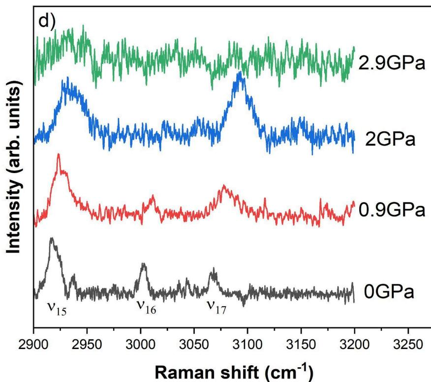
**Figure 7:** Raman spectroscopy spectra of sulindac at different pressures and room temperature in the range: a) 60 to 780  $\text{cm}^{-1}$ , b) 785 to 1319  $\text{cm}^{-1}$ , c) 1458 to 1950  $\text{cm}^{-1}$  d) 2900 to 3200  $\text{cm}^{-1}$
