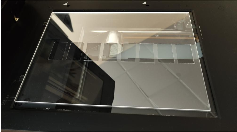
Figure 13: Template and acrylic glass for positioning the film on the scanner
