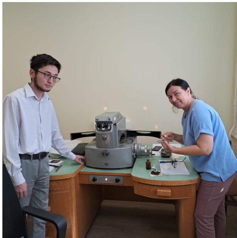
Fig. 9. Laboratory for measuring the ranges of short-range tracks of b-particles with KSM-1 optical microscope.
