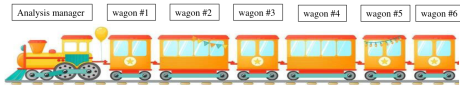
Figure 3.1: Sketch of the train analysis. Analysis manager reads event into memory and calls wagons one-by-one to modify and/or analyze data [35].
