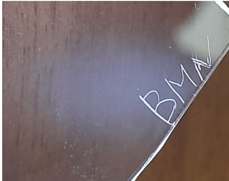
Figure 4: Appearance of the irradiated and etched area of SSNTD CR-39. The region of turbidity corresponds to the passage of the beam.
