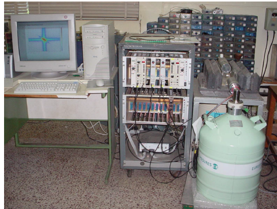
Figure 5: Doppler broadening measuring equipment available at the LEPTA project in JINR.
