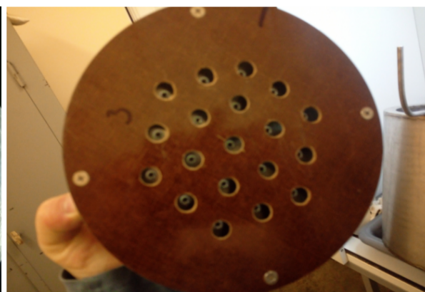
Pic. 16. Upper part of the dropper (view from below)
