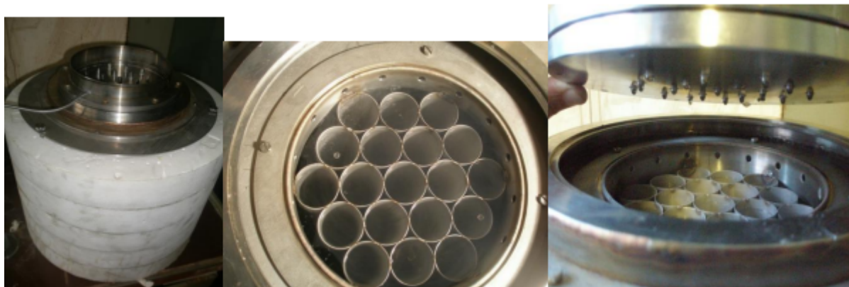
Pic. 14. Device for mass preparation of solid balls from a mixture of mesitylene and m-xylene: a general view of the device from the side, honeycombs with balls and a metal container with a dropper
