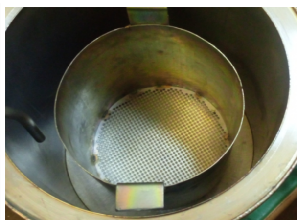
Pic. 20. Bottom screening mesh with a mesh diameter of 3.5 mm
