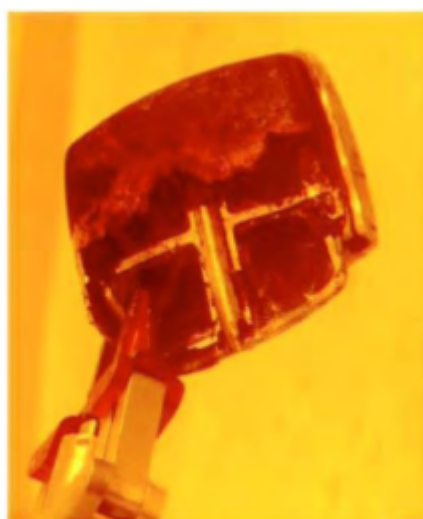
Pic. 35. Accumulation of deposits of tar and other formations in the moderator chamber after methane irradiation (b) compared to the new one (a)
