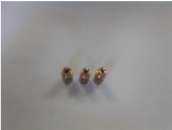
Pic. 29. Nozzles with a diameter of 2.5mm, from left to right 60, 90 and 120 degrees, respectively
