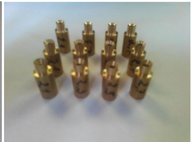
Pic. 30. Nozzles with a diameter of 2.1, 2.3, 2.5, 2.7 mm, bottom-up: 60, 90 and 120 degrees
