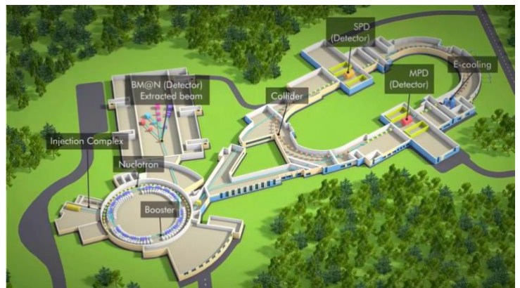
Figure 1: Schematic view of the NICA-Nuclotron complex and the position of the BM@N setup.
