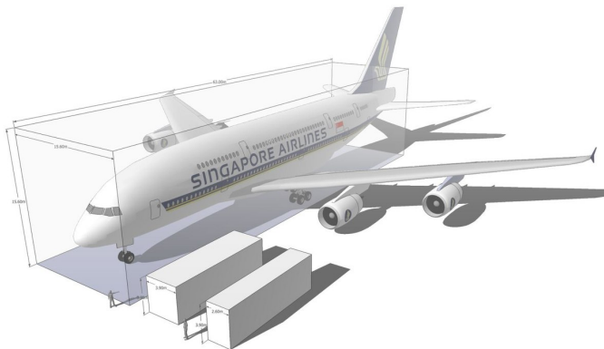
Figure 7: A comparison of the NOvA far and near detectors (and the NDOS test detector) with the size of an Airbus A380 and with an average human
