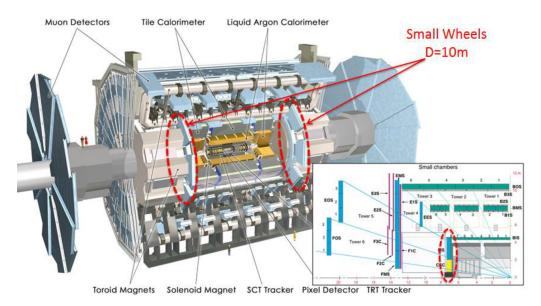
Figure 2: The ATLAS experiment at CERN.
