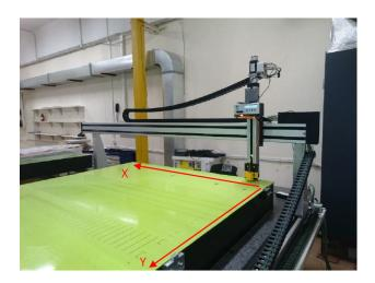
Figure 4: The optical probe measurement process on the vacuum tables.
