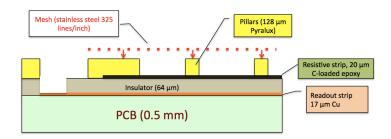
Figure 3: Internal structure of the Micromegas readout board and the placement of PCB.
