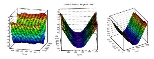
Figure 9: 3D fit and the three views of the granite table.
