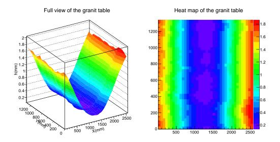
Figure 10: 3D fit and heat map of the granite table.
