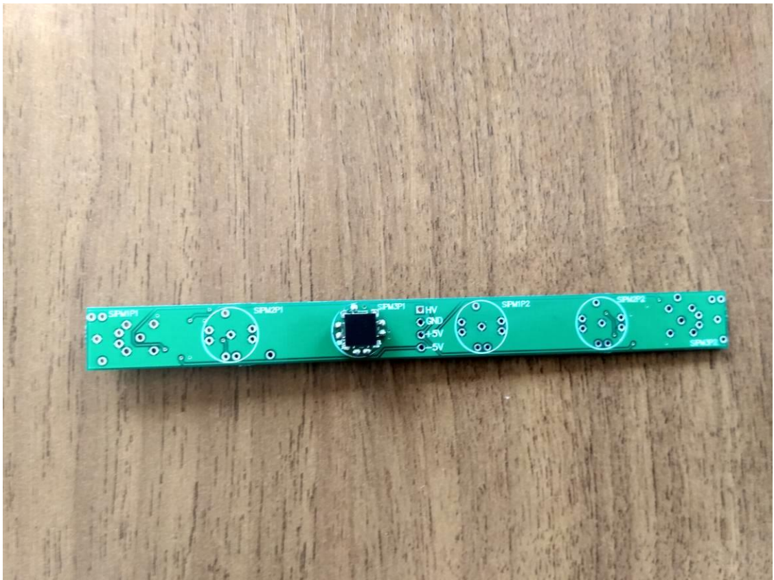
Fig. 7b. Lateral longitudinal plates with semiconductor photodetectors, side b.
