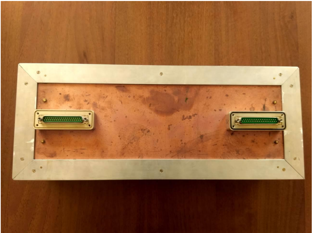
Fig. 1b. Experimental sample of a CMS Shashlik calorimeter prototype tower equipped with 25 aluminized WLS fibres, rear view
