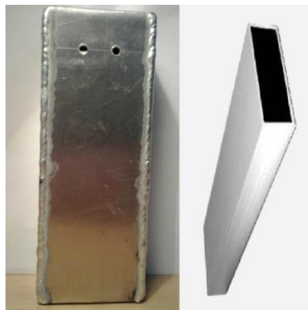
Figure 9. Cassette with a different value of thickness of the moderator (left – 4 sm, right – 2sm)
