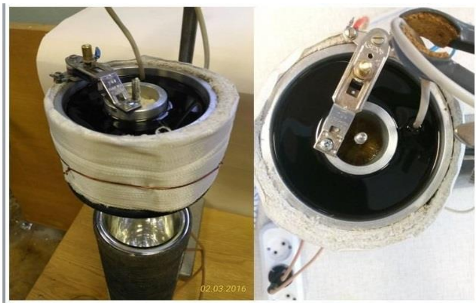
Figure 2. Facility for production of solid beads from triphenylmethane
