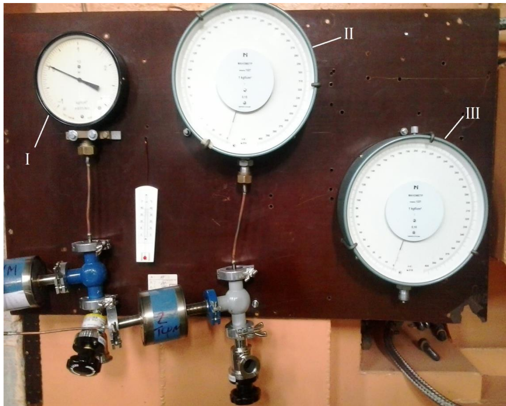
Figure 5. Pressure indications from manometers. (I - manometre with a mixture of mesitylene and m-xylene, II - manometre with powdery triphenylmethane, III - manometre with granular (pelletized) triphenylmethane)
