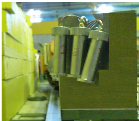
Figure 4. Samples before irradiation (I – ampoule with a liquid mesitylene and m-xylene, II- ampoule with a powdery triphenylmethane , III – ampoule with a beads from triphenylmethane)
