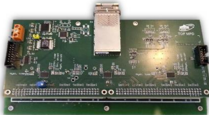
Fig. 3.2. 24-channel NINO based preamplifier board with the CXP output connector.
