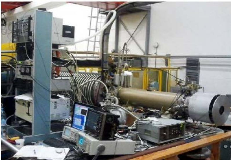
Figure 3.2 Krion-6T at high-voltage platform of LU-20 fore-injector. The Nuclotron Run #50.
