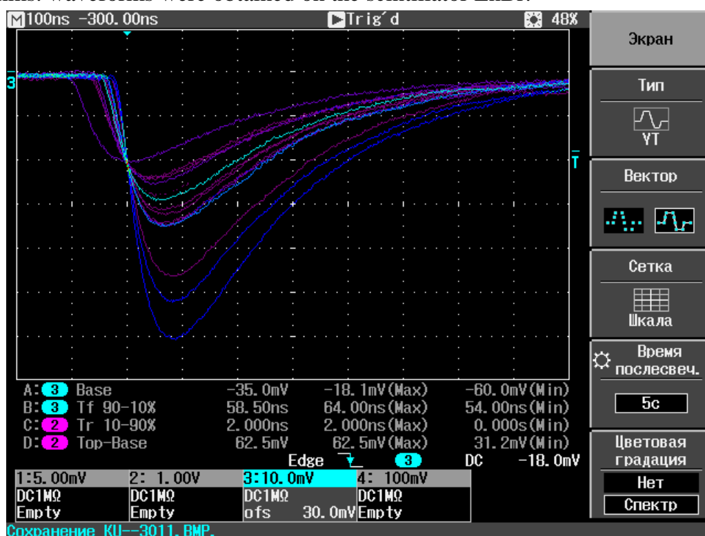
Figure 11. The output of the amplifier with a gain K \approx 3
