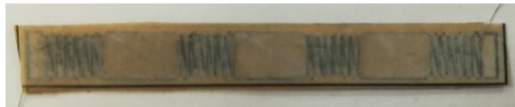
Figure 2. Heating element used in tests simulating four readout chips
