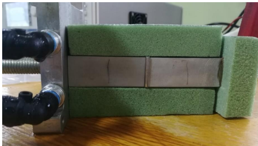
Figure 5. The test setup for measuring the thermal conductivity in a thin layer of adhesives.
