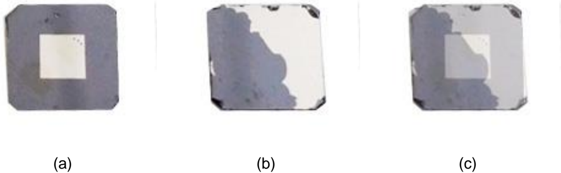
Figure 12. Photos of the studied detector: (a) input surface with the Ni anode (square shaped with light color), (b) exit surface with the cathode (irregular shape covering less than the half of the detector surface, light color), and (c) superposition of both images for comparison.
