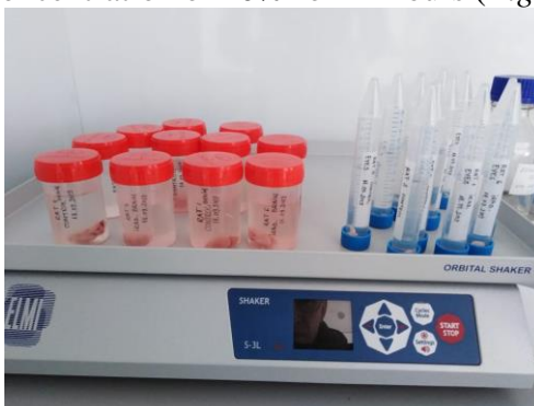
Fig.9. The specimen containers for the organs were filled with the formalin solution and placed on the ‘Orbital Shaker’ device
