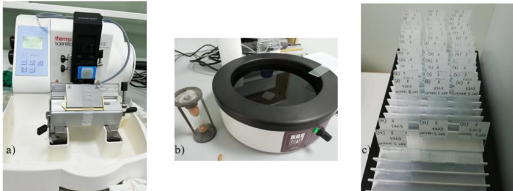
Fig.12. a) The device used for cutting slices (HM 340E semi-automated microtome), b) The warm water device in which the slices were placed, c) The final samples
