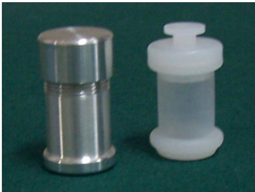
Fig 7 Transport containers used for irradiation: aluminum at the left and polystyrene at the right.
