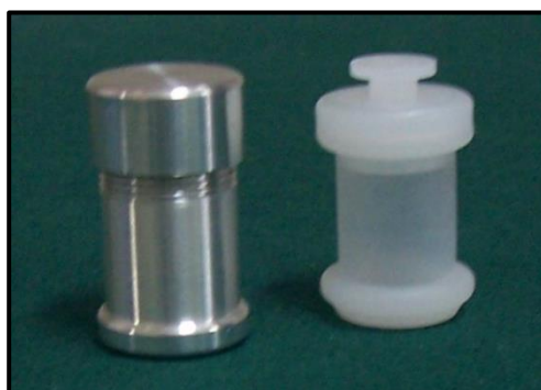
Fig.9. Transport containers used for irradiation: aluminum at the left and polystyrene at the right.
