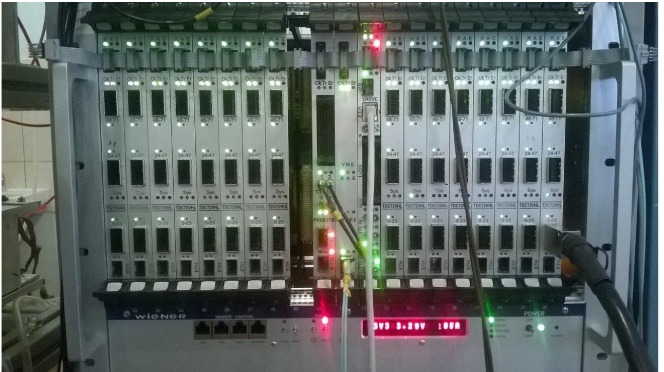
Fig. 6. VME crate with U40VE, FVME2 and 16 TDC72VHL modules
