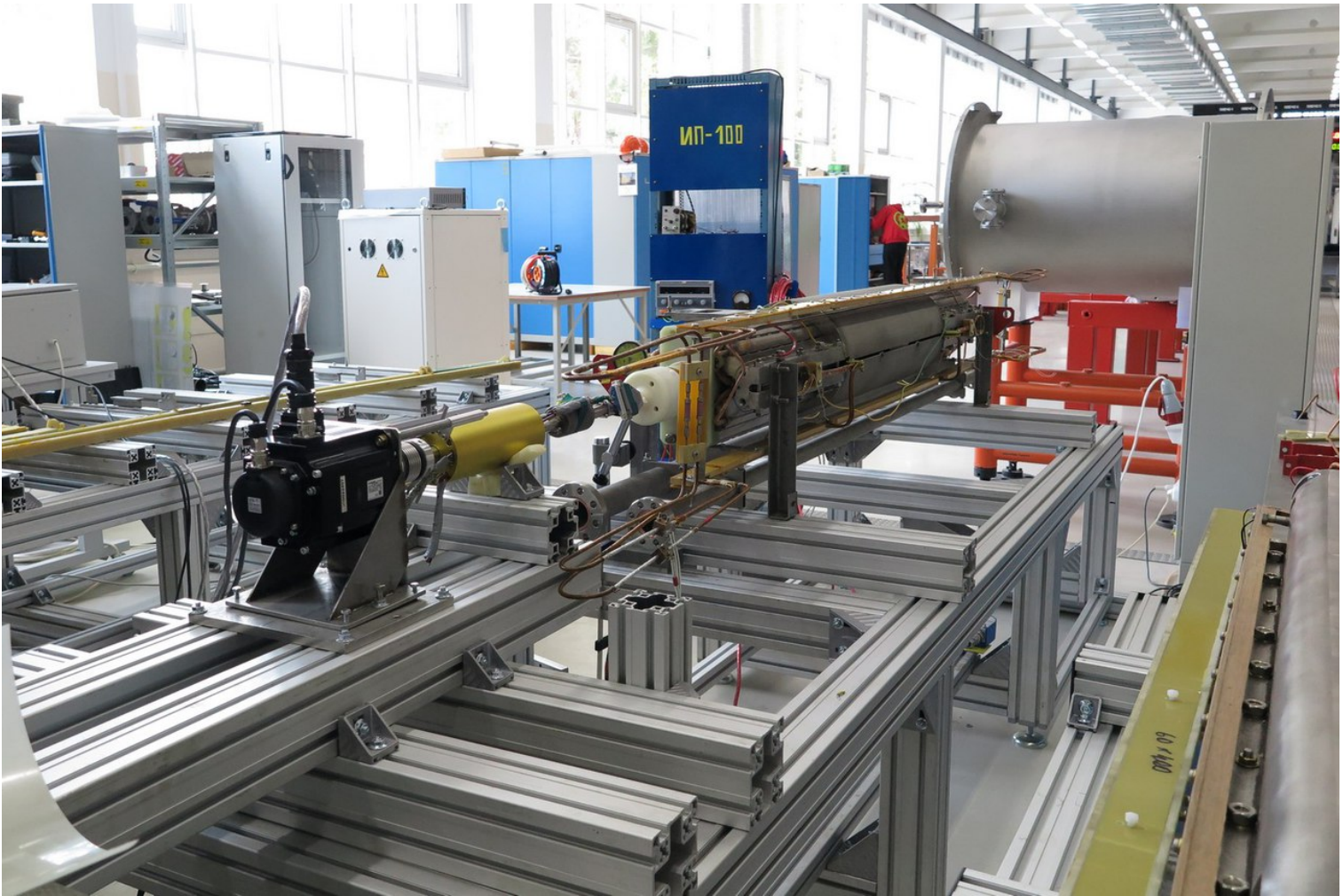
Fig. 17. The stand for quadrupole magnet
