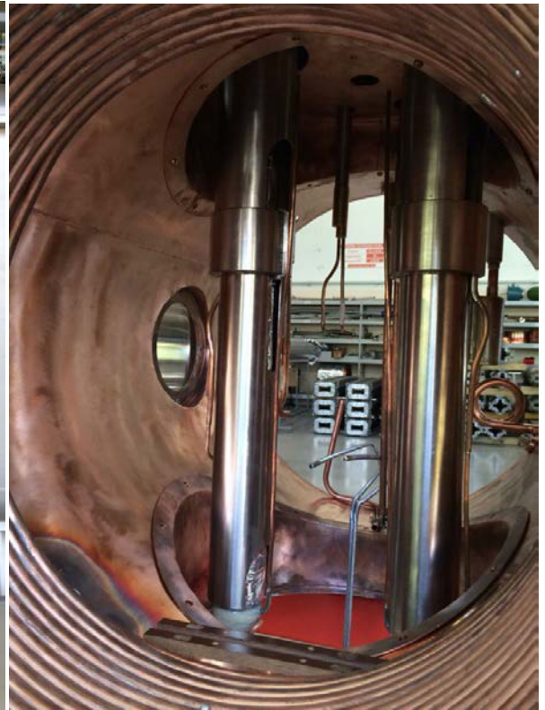
Fig.21. current leads the cryostat from the inside
