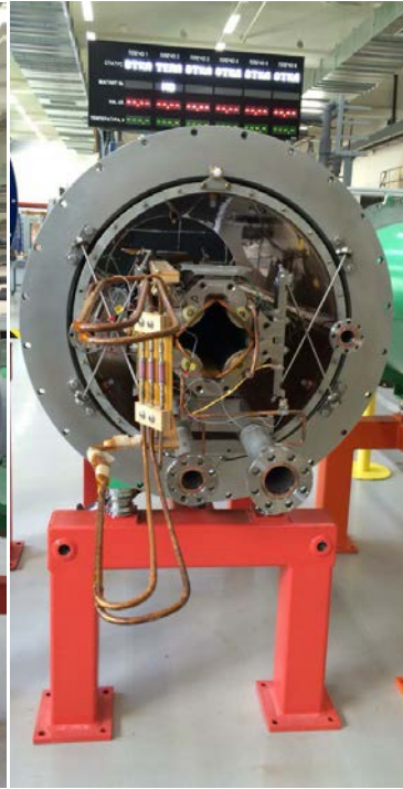
Fig. 3 Quadrupole magnets with multipole correctors for booster synchrotron
