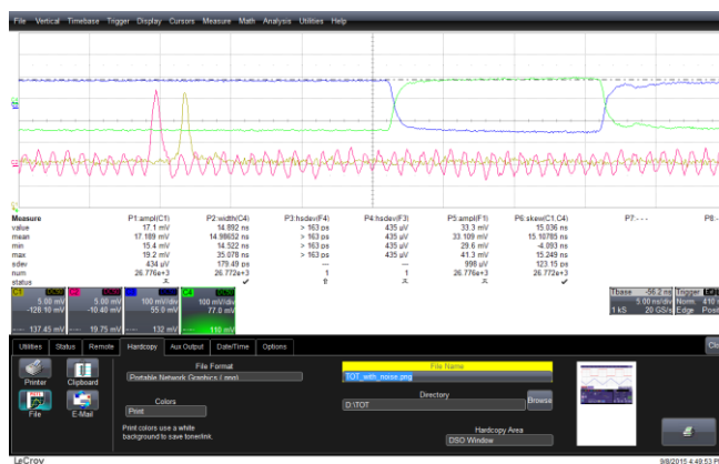
Figure 25 the different signals investigated: the primary signal without noise (yellow), the primary signal with noise (red) and the signals coming from the NINO amplifier (green and blue)
