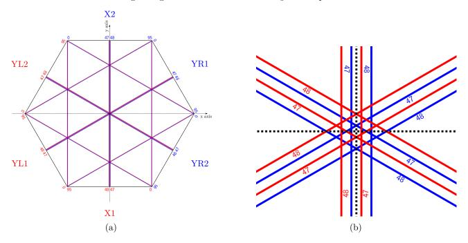
Figure 1: (a) Definition of the coordinate system with respect to the wire positions. Wire numbers are shown around the detector. (b) Close-up of the central region.
