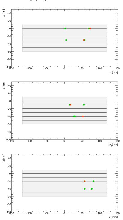
EVENT 195. An event with an impossible combination of  $\Delta i$  values. A three-dimensional straight line cannot be fitted well to these hits.
