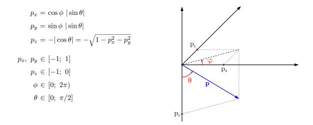
Figure 3: Definition of track parameters
