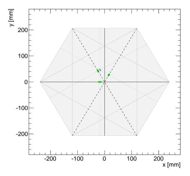
Example YX projection of a good event. Green dots represent averaged location of a good hit in each plane. The dotted grey lines represent averaged locations of good hit wires in the top three planes, whereas the dashed grey lines correspond to the three bottom planes. The fitted track is drawn in blue. The event 21, which is shown in this figure, has only one hit in each plane, thus the hit locations are exact.
